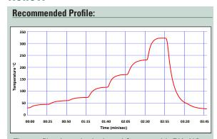
The profile above is designed for use with BiAgX $\circledR$  in a nitrogen atmosphere or forming gas (<100 ppm O2). It can serve as a general guideline for establishing a profile for your process and should be regarded as a typical example. Adjustments to this profile may be necessary based on assembly size, thermal density, and other factors.
