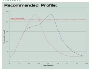
A short preheat  $(150^\circ-160^\circ\text{C})$  for less than 45 seconds may be used to reduce voiding. The profile should ideally be a linear ramp at  $1-2^\circ\text{C/second}$  up to  $20-30^\circ\text{C}$  above solidus temperature, with a rapid cool down afterwards, and a minimum time above liquidus of 20 seconds.
